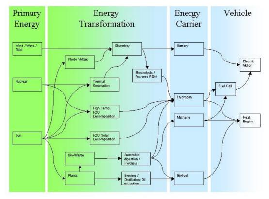
Each brings different issues making them more or less viable. For example battery technology is gradually improving but energy densities are still far below that provided by (say) petrol. Fuel cell vehicles could run off 'traditional' fuels such as Methane (as in natural gas) or hydrogen. Both of these require
